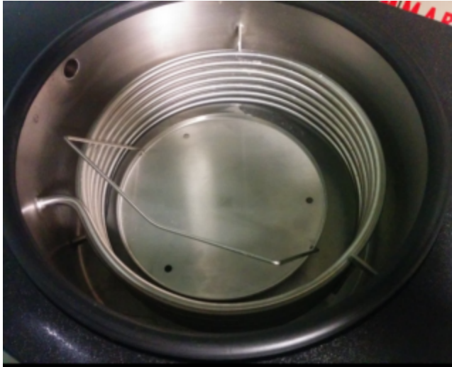
baffle plate and condenser coil inside the chamber
